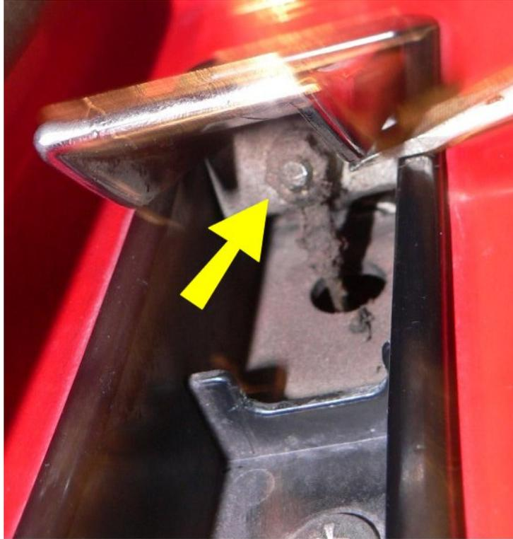
3. Lift latch & remove the 8mm nut & lock washer holding the cable eyelet to the latch-lever.
