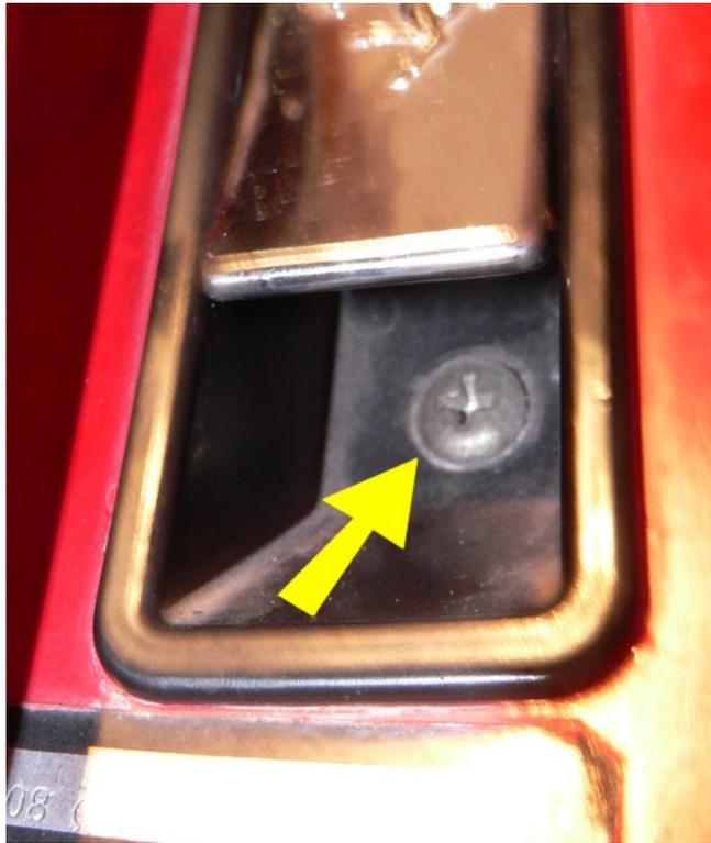
5. Remove the #2 Philips screw that attaches the latch housing to the body.
