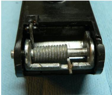
10. Clean old grease off of the latch-lever, spring, & hinge pin. Also wire brush the cable mounting stud's threads to remove any corrosion.
